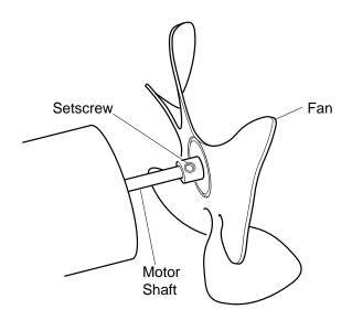
Figure 21 - Fan, Motor Shaft, and Setscrew Location
